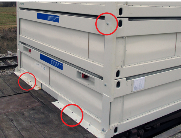
Modular units needs to be fixed with metal profiles to prevent modular units from sliding.
