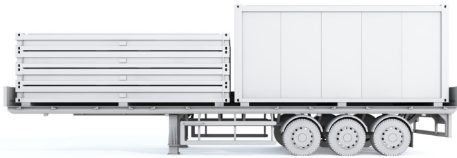
Truck transport of flat-packed/assembled modular units without forklift openings*
