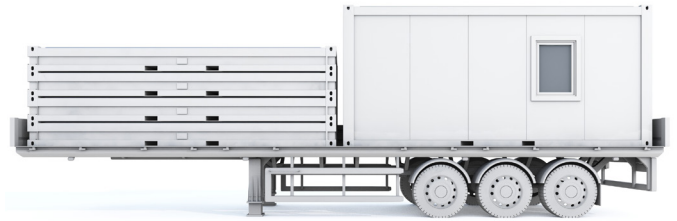
Truck transport of flat-packed/assembled modular units with forklift openings*
